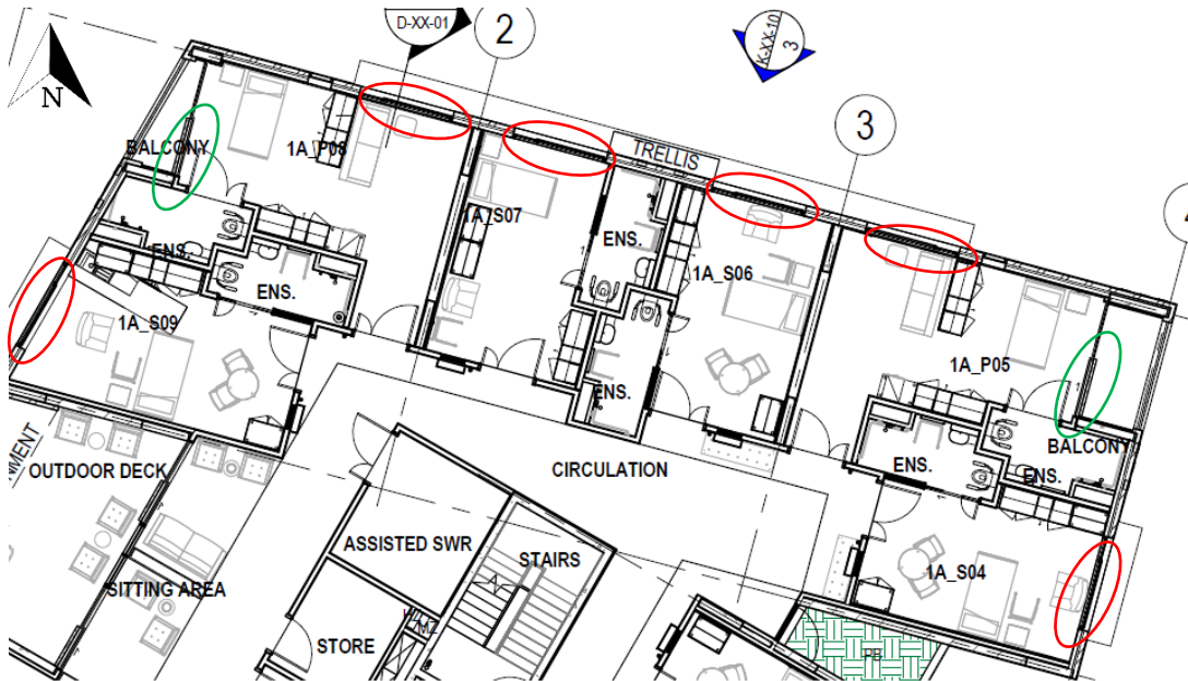
Figure 4 Detail of test rooms, showing combination windows (red) and sliding doors (green)
